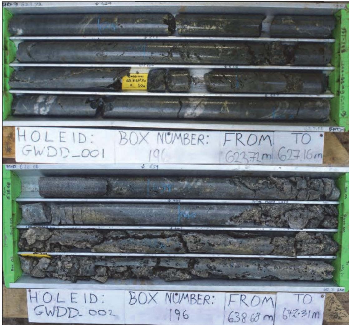
Figure 10.3: Core Photos of Semi-Massive Sulphide Mineralisation in Cornish Lithium Drill holes GWDD-001 and GWDD-002
