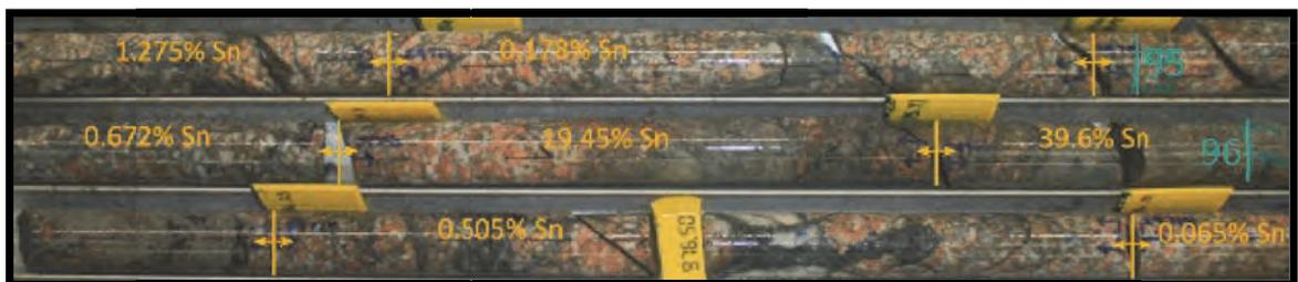
**Figure 24.1: No. 4 Lode Mineralised Intercept in SDD20\_001B between 1,034.38m and 1,035.59m down hole**
