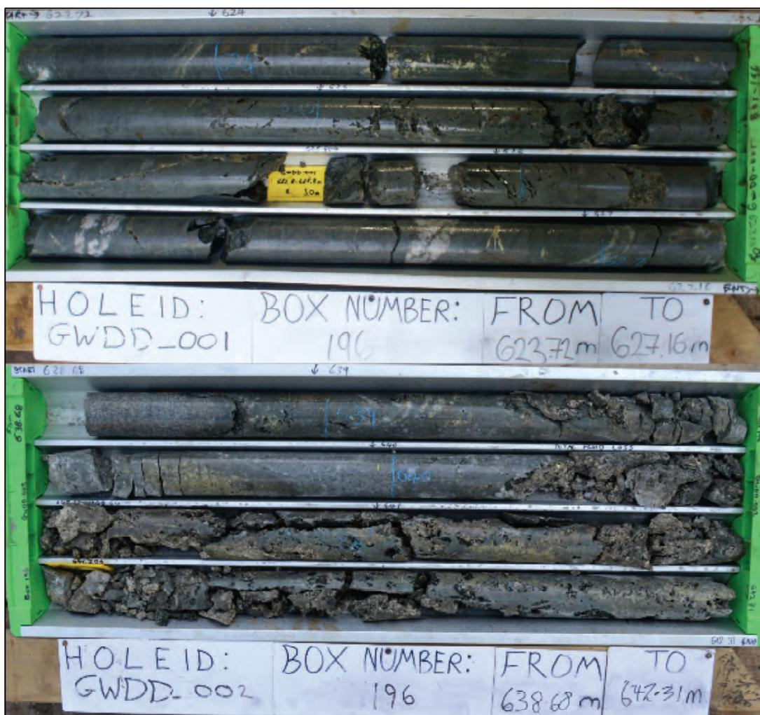
Figure 12: Core photos of semi-massive sulphide mineralisation recovered in drill holes GWDD-001 and GWDD-002
