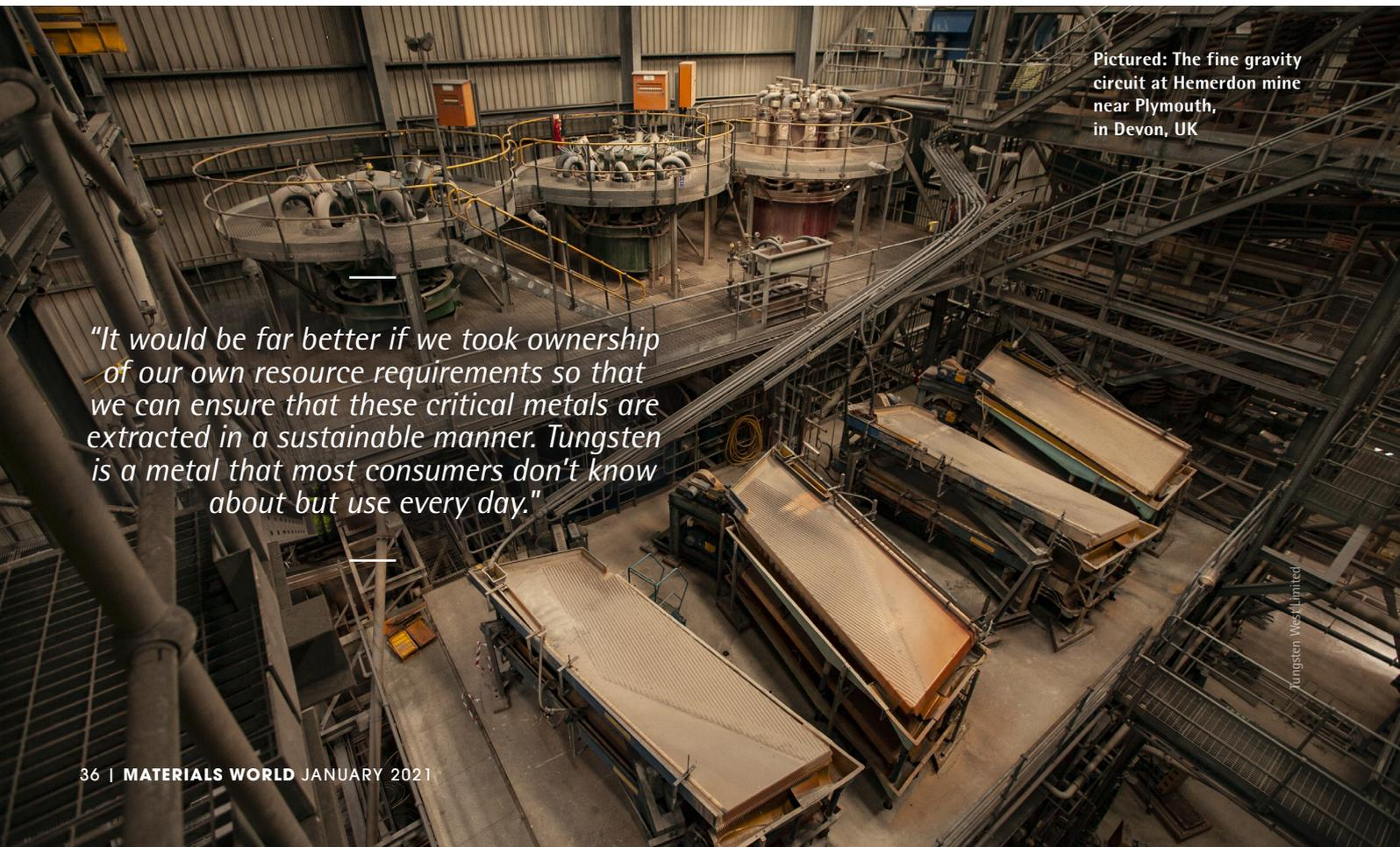
Pictured: The fine gravity circuit at Hemerdon mine near Plymouth, in Devon, UK
